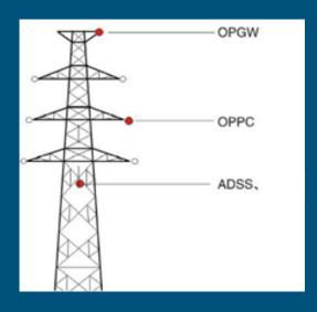
All Dielectric Self Supporting cable (ADSS) has no metallic parts. It can be placed in the electric space. It is also much lighter. VELCO figured they could use ADSS fiber with 72 strands as it does not materially impact pole loading. Optical Ground Wire (OPGW) has fiber in the core of the top conductor of transmission towers, Optical Phase Conductor (OPPC) has fiber in the core of the power line itself.
