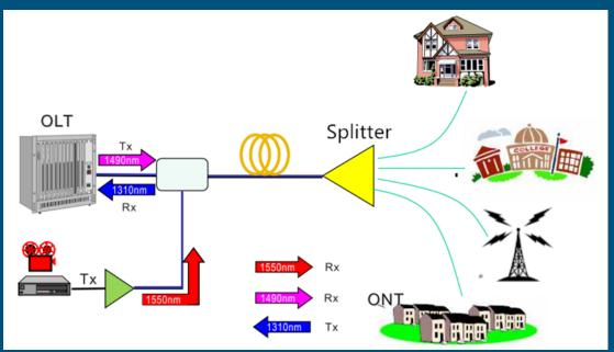
The start of the network is the optical line terminal **(OLT)**. It converts the traffic in the carrier's internal backbone network to the optical wavelengths and framing structure used by the Passive Opt Network (PON).
