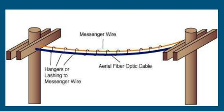
Most traditional telecommunication installations hang fiber from a messenger (steel cable). That cable has to be 40" away from the lowest electrical conductor. The steel messenger adds weight to the pole, which can result in pole change-outs. These change-outs are very expensive.
